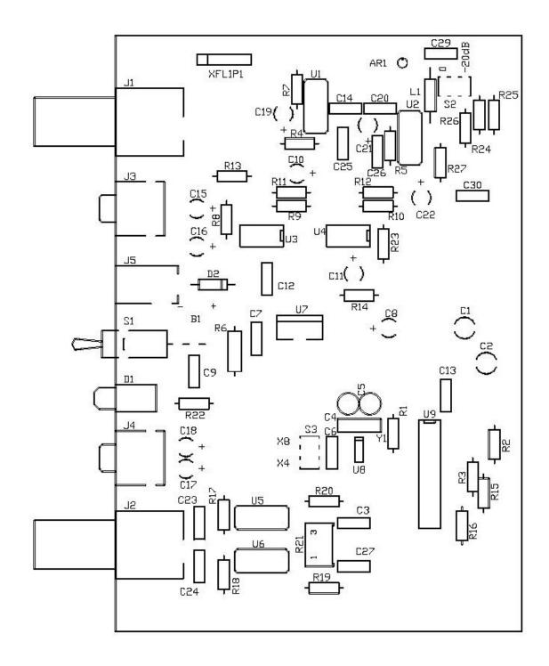
Build the band pass filter board and plug it into the main board, with the solder side facing the edge of the main board.
