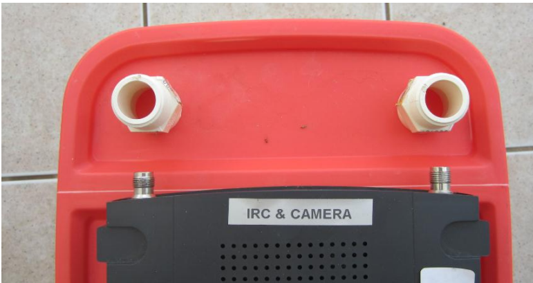
Alignment of whip antenna holes
