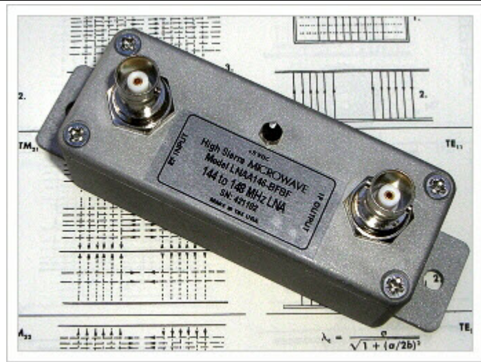
Picture shows the BNC female input and output option: "XXXX" = "BFBF"
