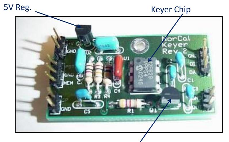
Output Transistor (to key rig)
