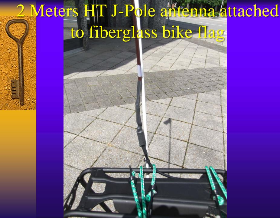
J-Pole antenna attached to bike flag, but ended up trimming 6" on top
